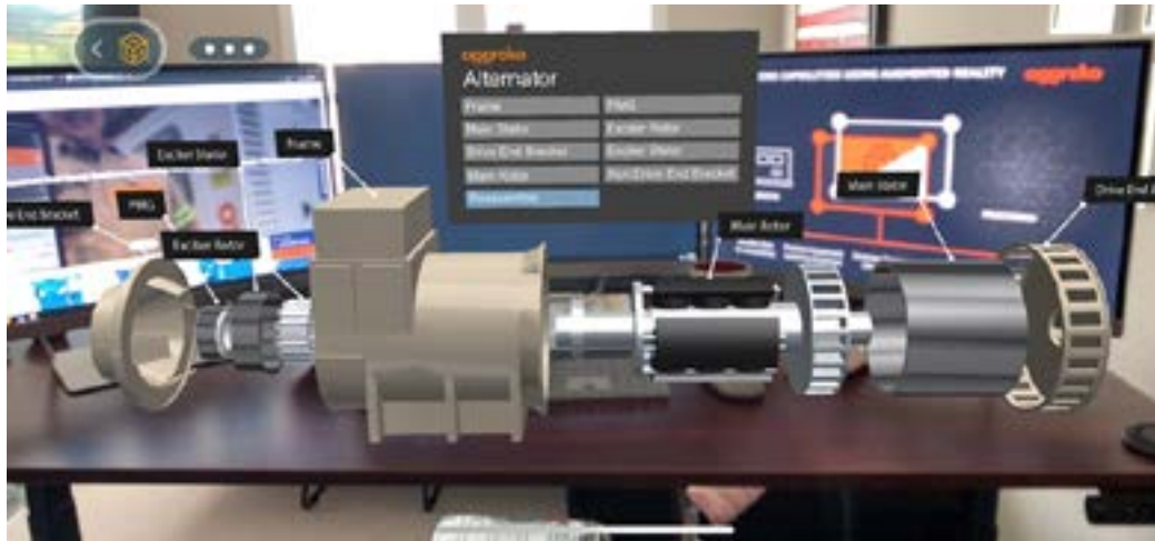
Alternator parts and components activity used during Aggreko Alternator & Schematics virtual course using ScopeAR Worklink
